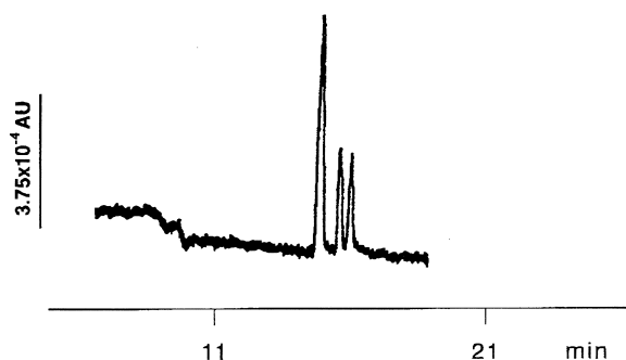
Fig. 4. Chiral separation of labetalol (11) by the counter-EOF setup in aqueous CE. Buffer: 2.31 w/v% (~15 mM) \beta -CD-(SO 4 - ) 4 in 50 mM Tris–citrate (pH 5.11). Field strength: –357 V/cm.
